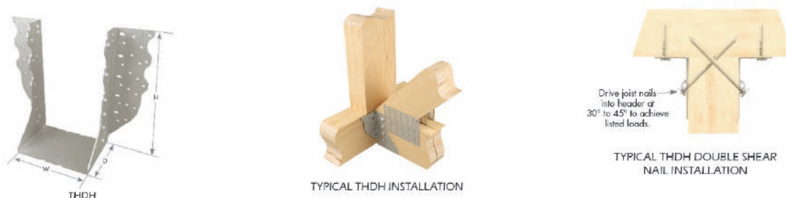
FIGURE 9—THDH FACE MOUNT HANGER
