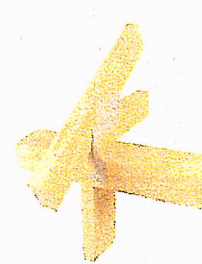
Typical RT7 truss/rafter to double plate installation
