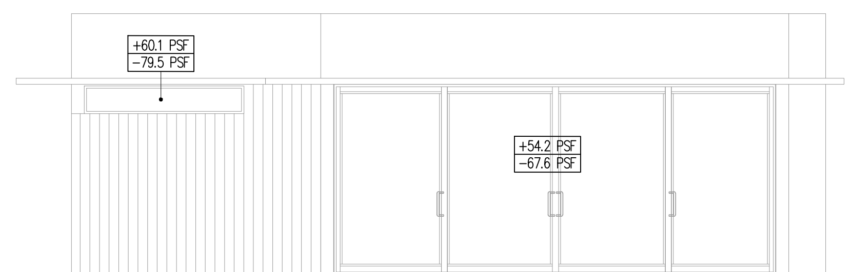
DESIGN WIND PRESS. - EXT. DOORS & WINDOWS SOUTH ELEVATION - GUESTHOUSE
