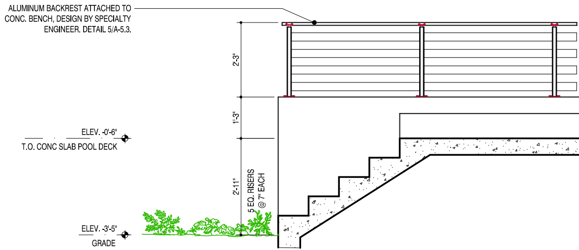
ENLARGED SECTION STAIRS B 1 0 1 2 3 4 SCALE: 1/2" = 1'-0"
